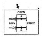
PLUG INTO THE LOWER SOCKET BREAKS THE LINK ... (SAME AS NORMALLED) PARALLEL:
